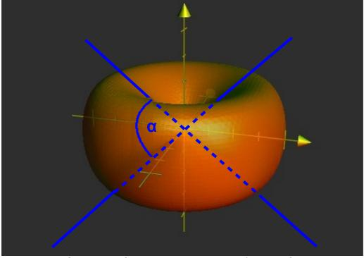
The outer surface area of the ring is about:  $\alpha/180^{\circ} \times (4 \pi r^2)$ = 1/1.64 (4  $\pi r^2$ ) for dipole antennas.
